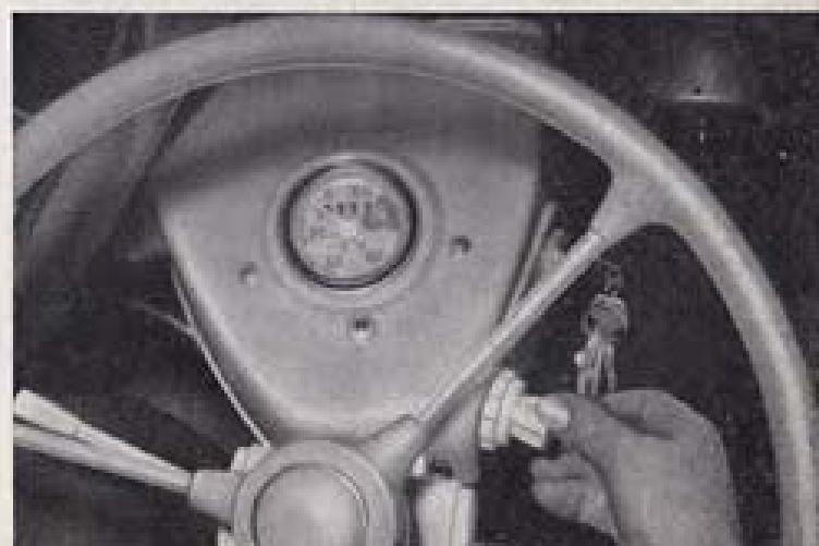
leaving the steering wheel (**figure 11**). To bring the wiper motor in motion, operate the switch of this unit, fitted to the door beside the instrument panel (**figure 12**), and finally let us mention the seat adjustment procedure. Having removed the covering board below the seat, you may slacken the two hexagon screws and adapt the seat to your requirements (**figure 13**). For the other controls and instruments see figure 1 page 17.
