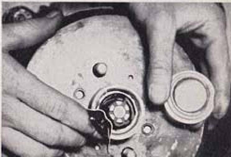
ball bearing grease into the bearings. Under no circumstances fill the dust cap completely and replace because such a procedure may inject grease into the brake linings (**figure 45**). For the detailed indication of the prescribed maintenance jobs and the corresponding service periods see attached Maintenance Survey (**page 56 and appendix**).
