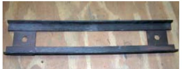
If I was making this over again, I would use (1) 3" x 15" x 1/8" plate on the bottom frame instead of the (2) 2" x 3" plates. I have found that the opening in the bottom of the frame hinders its operation.
