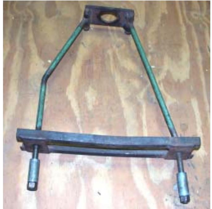
The top plate is 2-3/4" wide x 5" long x 1/4" thick. It has a hole in the middle 1-3/4" in diameter. This hole secures it to the spring housing and keeps it from slipping off when being used.
